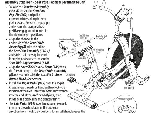
tighten firmly with the 6mm Hex Wrench. Select a suitable space for operation of the AirBike Elite. Move the unit to the desired location by raising the rear stabilizer off the ground until the transport wheels touch the ground. Slowly push the unit into place. Ensure there is 0.5 m (19.7 in.) of clearance on all sides of the bike.
