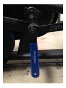
**Step 2:** Once the Crank Fixing Bolt is removed (part#42) is removed install the crank puller. Use the crank puller to remove the Crank Arm (part#18).
