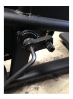
**Step 4:** To remove the Bell Crank (part#40) use the 8mm hex wrench to rotate the Crank Fixing Bolt (part#42) counterclockwise until it comes off.
