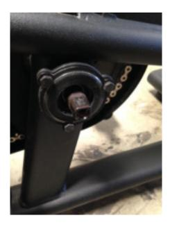
**Step 6:** Once the old Bell Crank (part#40) is removed install the new one.
