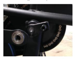
**Step 3:** After removing the crank arm remove the Linkage Arm (part#12) exposing the Bell Crank (part#40). When the Linkage Arm is removed also remove the thin plastic washers that are between the Linkage Arm and the Bell Crank. Your unit may or may not have the plastic washers.
