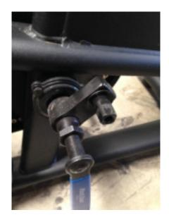
**Step 5:** After the Crank Fixing Bolt (part#42) is removed install the crank puller and then remove the Bell Crank (part#40).
