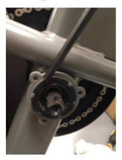
**Step 2:** Using the Allen wrench or the flat screwdriver tap the Bottom Bracket Lock ring **counter clockwise**.
